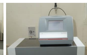
Microwave Synthesizer (Monowave 200, Anton Paar)
